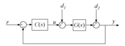
For 2-DOF PID controller types such as PI2, PIDF2, and I-PD, **PID Tuner** computes responses based upon the following architecture:
