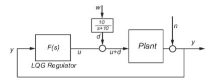
The goal is to regulate the plant output y around zero. The input disturbance d is low frequency with power spectral density (PSD) concentrated below 10 rad/s. For LQG design purposes, it is modeled as white noise driving a lowpass filter with a cutoff at 10 rad/s, shown in the following figure.
