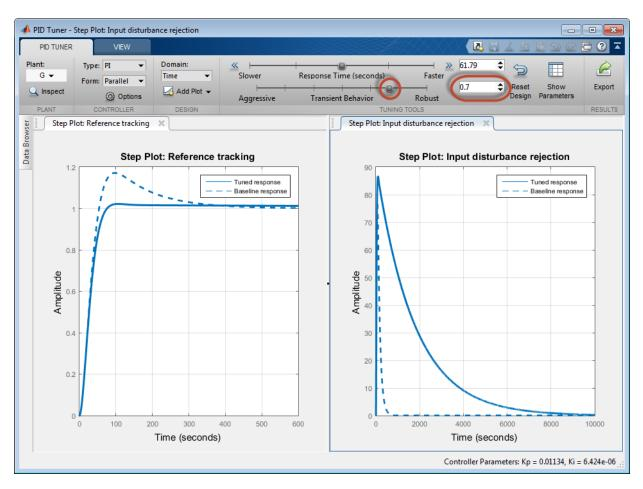
Increasing the transient-behavior coefficient to 0.70 nearly eliminates the overshoot, but results in extremely sluggish disturbance rejection. You can try moving the **Transient behavior** slider until you find a balance between reference tracking and disturbance rejection that is suitable for your application. The effect that changing the slider has on the balance depends on the plant model. For some plant models, the effect is not as large as shown in this example.
