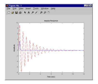
**Comparison of Open- and Closed-Loop Impulse Response**
