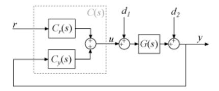
The system responses are based on the decomposition of the 2-DOF PID controller, C, into a setpoint component Cr and a feedback component Cy, as described in "Two-Degree-of-Freedom PID Controllers".
