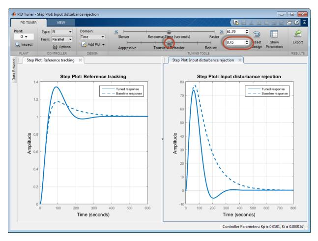
Lowering the transient-behavior coefficient to 0.45 speeds up disturbance rejection, but also increases overshoot in the reference-tracking response.
